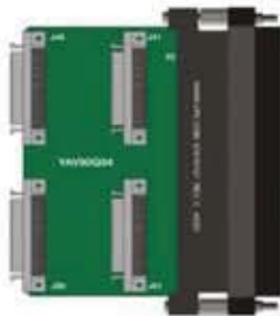
YAV90Q04 6200.54 4x I DC 50 to Quadrapaddle 192 pins Interface
