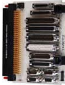
YAV90TC2 6200.37 Connectors Interface to VPC 90
