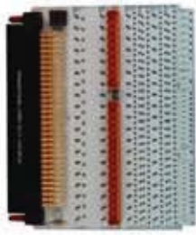
YAV90TC1 6200.36 Terminal block sockets interface to VPC 90.
