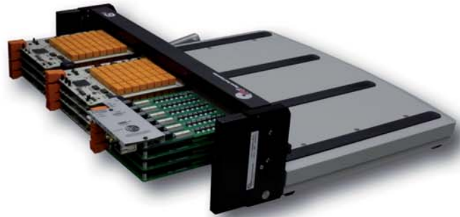
ATE Mass interconnect full of 6TL modules
